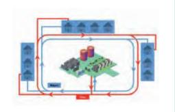
Underground pipes then deliver hot water or steam around a central closed loop system. When you use the heating or hot water, the system in your house will draw hot water from this system and, in turn, heats the water in your property. It does this through a Heat Interface Unit (HIU) which is installed in your kitchen instead of a boiler (see below for more information regarding your HIU).
